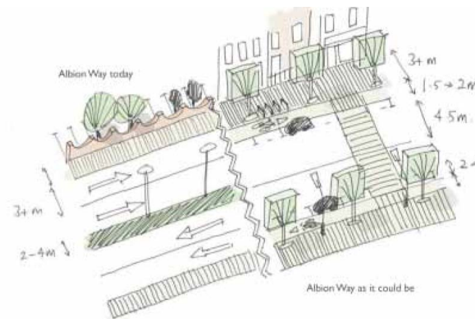
Horsham Town Plan shows how a cycle track can pass behind parked cars
