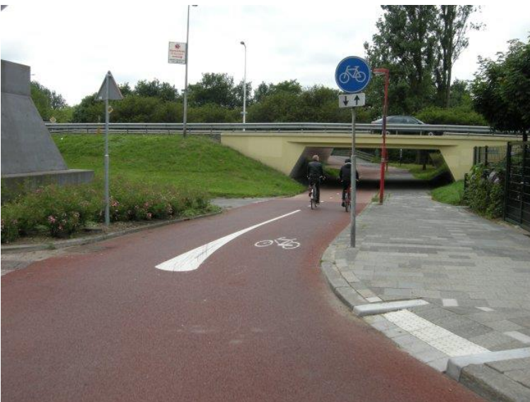
Cycle underpass with good open aspect, gentle slopes and a separate footpath (Picture: Mark Treasure)
