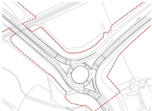
Figure 5.9: A264 / B2195 (Moorhead) Junction Potential Capacity Improvements
