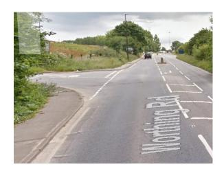
Signalised junction for the Park and Ride –a fast two lane approach from both directions. It is hazardous for cyclists and lacks any specific cycling infrastructure.
