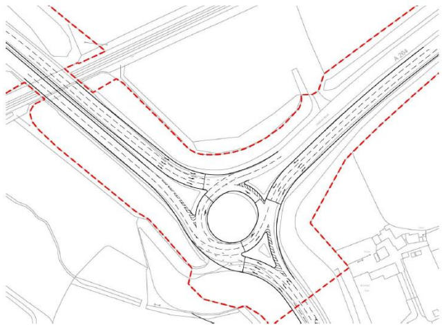
Figure 5.9: A264 / B2195 (Moorhead) Junction Potential Capacity Improvements
